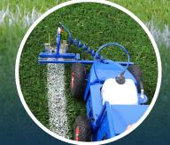
RDS Slide rail provides variable line position providing operator choice of comfortable spray head positions.
